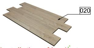
installation of laminate parallel to the main entrance in a single array in the rooms 2, 3, 4,8,9,10,11
